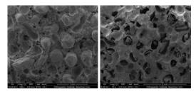
*Fig. 1: SEM images of the Mg-PMMA bone cement (left) before degrade and (right) after degrade.*
