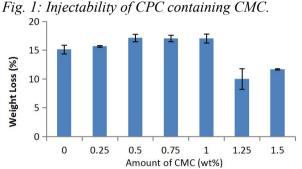
Fig 2: Weight loss percentage attributed to the washout effect of a CPC containing CMC.
