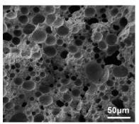
Fig. 1:SEM image of the fracture surfaces of Si-HPMC foamed CPC injected into a saline solution immediately after preparation  $(L/P_{total} = 0.8, V_{air}/V_{hydrogel} =$ 1.0).
