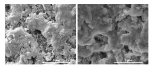
Fig. 1: SEM images of the SF CPCs (left) and tSF CPCs (right).
