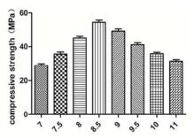
*Fig. 1: Compressive strength of CPCs at different pH of tSF solution (SF group: pH=7).*
