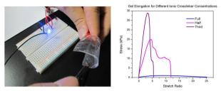
Fig. 1: (a) Full gel sample conducting electricity to illuminate an LED. (b) Stress vs. stretch ratio graph showing elongation of all three samples until fracture.
