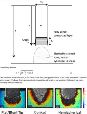
Fig 1. (Top) Extract of our mathematical model for the cracking and compaction of osteoporotic bone Fig 2. (Bottom) Strain fields of various implant tips in osteoporotic bone specimens.
