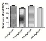
*Fig. 2: Compressive strength of Mg-PMMA bone cement*
