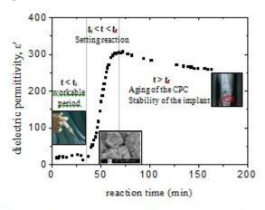
Fig. 1: Variation of dielectric permittivity, ε' versus reaction time for the undoped CPC.
