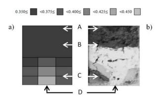
Figure 1: a) LPR distribution remaining in syringe barrel post injection. Key value represents LPR; b) Cutaway view of powder remaining in syringe barrel for an initial
