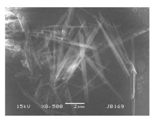
Fig. 1: SEM micrograph of CaP nanowires.
