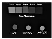
Fig. 1: Radiopacity of Sr substituted CPCs.
