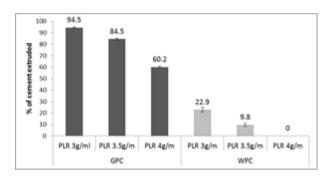
Fig. 1: Percentage of extruded GPC and WPC using 19G stainless steel needles. Fig. 2: Influence of PLRs on the compressive strength and porosity of GPC and WPC.
