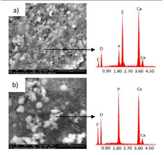
Fig. 1: SEM and EDS images of the cement A4: a) non-incubated, b) incubated in SBF for 7 days.
