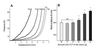
Mechanical tests were highly dependent on the number and the spatial distribution of macropores. The granules with the lower amount of  $\beta$ -TCP were the most porous and were the more friable. On the contrary, the 25g denser granules exhibited the highest compressive energy (Fig.2).
