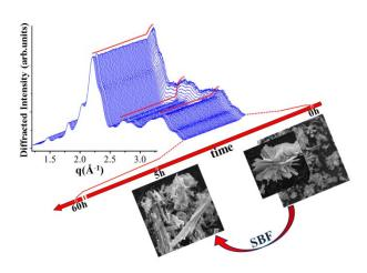
Fig. 1: 3D Map of the EDXRD patterns collected upon the OCP-DCPD-SBF system. Diffraction data are complemented with the SEM results.
