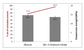
Fig. 1: Effect of Calcium nitrate on the extrusion and compressive strength of EB.
