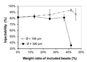
Fig. 1: Injectability of pastes vs. weight ratio of included beads (B diameters = 156µm or 390µm)
