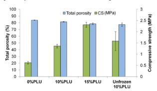
Fig.3: Total porosity and compressive strength of Pluronic containing CPFs, and unfrozen CPF.
