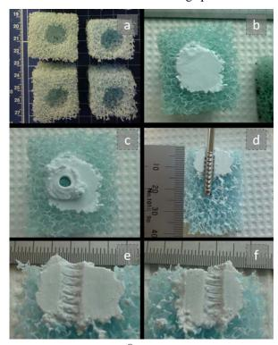
Fig. 1: a) SAWBONES® blocks with created voids, b)Void filled with CERAMENT<sup>TM</sup> /BVF, c) Drilled sample, d)Illustration of placement of screw through the cement, anchorage in foam, e & f) Cross-sections of drilling channel
