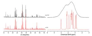
Fig. 1: XRD data and  $^{31}P$  MAS NMR data for  $\alpha$ -TCP ( $Ca_3(PO_4)_2$ ) (bottom), and Si- $\alpha$ -TCP ( $Ca_3(PO_4)_{2-x}(SiO_4)_x$  (x=0.10)) (top).
