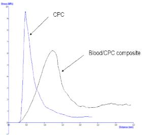
**Figure:** Comparative compressive strength tests for CPC and blood/CPC composite.
