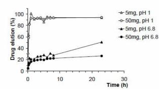
**Fig.1**. Elution curves for cements containing 5 and 50mg of the drug in an acid solution (pH=1) and a buffer solution (pH=6.8)
