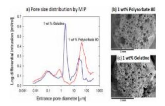
**Fig.1**: a) Pore size distribution obtained by MIP for the Polysorbate 80 and gelatine CDHA foams; b,c) respectively Polysorbate 80 and gelatine CDHA foam macrostructure. In all cases the quantity of the foaming agent is 1 wt%.
