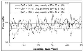
Fig.2: Local porosity versus x-position of layers; samples were produced at sintering tem. of 1000  $^{\circ}C$ .
