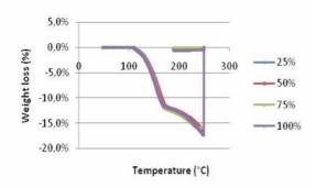
**Fig. 2** Weight loss as a function of the percentage of injected cement (on 4 ml)
