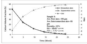
Fig.1: Exponential series approximation of the simulation results and resorption rate data
