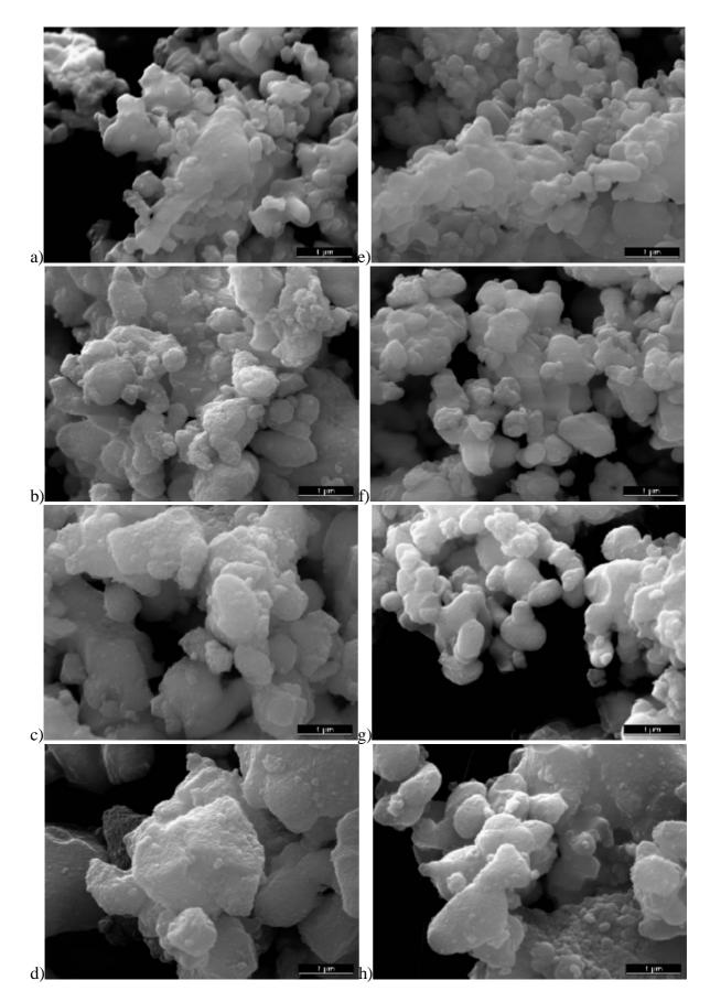
*Figure1* SEM pictures (20'000x): a) 1-step, 850°C, Ca/P=1.475; b) 2-step, 850°C, Ca/P=1.475; c) 2-step, 900°C, Ca/P=1.475; d) 2-step, 950°C, Ca/P=1.475; e) 1-step, 850°C, Ca/P=1.5; f) 2-step, 850°C, Ca/P=1.5; g) 2-step, 900°C, Ca/P=1.5; h) 2-step, 950°C, Ca/P=1.5.
