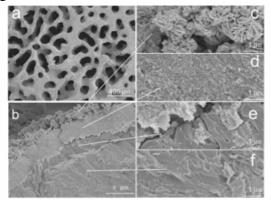
**Fig 1.** SEM Electronic micrographs of the surface structure of the CHACC cross-sections. (a) low magnification of CHACC. c-f shows sequential crosssections from b. (c) the surface crystalline HA, (d) a 5-10 $\mu$ m adjacent layer, (e) a junction between layers and (f) inner core structure.
