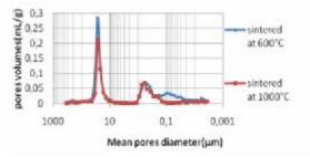
**Fig. 1** Pores Volumes and mean pores diameter as a function of sintering temperature
