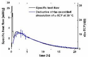
**Figure 1**: Derivative of the dissolved  $\alpha$ -TCP with respect to the time and the correlated specific heat
